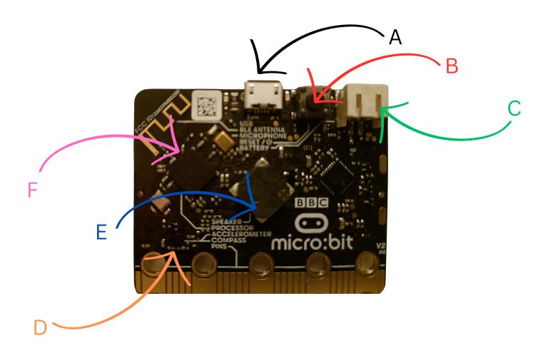
A- This is the part that you plug the USB wire into which allows you to download code onto your Microbit.
